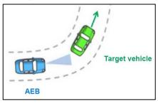
When driving on a large curve road, due to the sensor limitation, collision with the front vehicles or other objects may occur.
