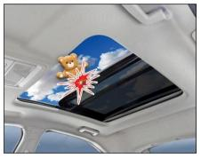
If the sunroof senses any obstacle while it is closing then it will reverse its direction and opens the sunroof so that trapped object will get released easily. The auto reverse function may not work if very thin or soft object is caught between the sunroof assembly. Anti-Pinch/ Automatic reversal is a safety feature however to override it and operate sunroof manually, press sunroof close switch within 10 seconds of auto-reversal completion and hold it till sunroof is fully closed.
