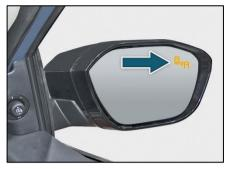
Level 1 Warning: (Object detected in the BSD-LCA zone): The warning light on the ORVM will be continuously ON.
