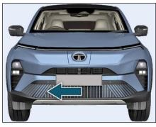
Outside Ambient Temperature (OAT) sensor located under the front bumper grill.
