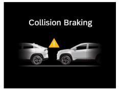
When Only FCW is ON, the system gives only one level of warning. The driver is alerted to the risk of an imminent collision by visual and audible warning which may be accompanied by a short brake pulse.
