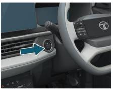
Single press start/stop switch will bring the vehicle to the ACC ON condition (Amber color)
