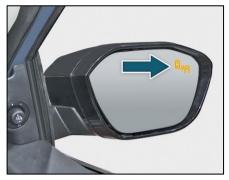
Level 1 Warning (Object detected in the zone): The warning light on the ORVM will be continuously ON.
