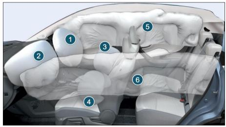
The SRS [Supplementary Restraint system] is designed to provide protection to occupants in case of collision or sudden impact, when crash is detected, the SRS airbag system deploys airbags to help reduce the risk of injury to the occupant. It works in conjunction with seat belts. There are 6 airbags provided in your car:
