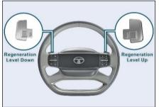
By using the regeneration switch (Pull type) driver can Up/Down regeneration level.
