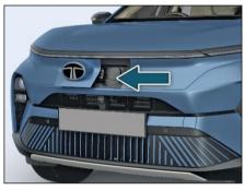
Before connecting the charging gun to vehicle charging socket, make sure the gun lock is released.
