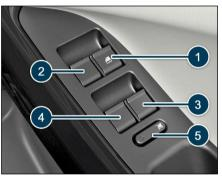
Window glasses 1-2-3-4 on all four doors can be operated by switches provided on the main control panel located on the driver's arm rest. They work only when the key is in the 'IGN ON' position.
