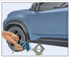
Continue to raise the jack slowly and smoothly until the tyre clears the ground. Do not raise the vehicle more than necessary.
