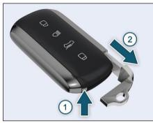
Press the knob (1) to release the key. Pull the key blade (2) out.
