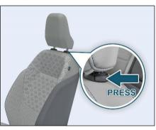
Adjust the head restraint so that it is as close to the head as possible and center of the head restraint supports the back of the head at eye level.
