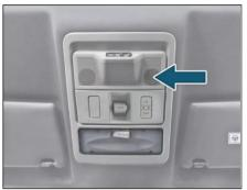
Mic is provided near the roof lamp.
