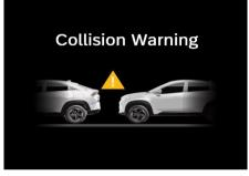
1st Warning - The driver is alerted to the risk of an imminent collision by visual and audible warning which may be accompanied by a short brake pulse.
