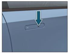
Push the handle slightly at the area on the Gripper as shown in the image.
