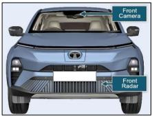
Front ADAS features uses front radar and front windshield camera, as shown in above image.
