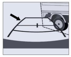
Visually check the surroundings and the area behind the vehicle. In the case shown below, the truck appears to be outside of the vehicle width guidelines and the vehicle does not look as if it hits the truck. However, the rear body of the truck may actually cross over the vehicle width guidelines. In reality if you back up as guided by the vehicle width guidelines, the vehicle may hit the truck.
