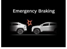
2nd Warning - If the driver does not take action or the driver braking force is not enough to mitigate collision, system issues the second level of visual and audible warning and applies emergency braking.
