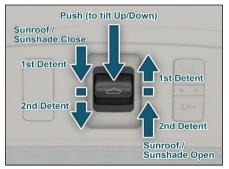
Power sunroof switch is mounted in overhead console near the roof lamp. This switch is used to open, close, tilt up / down the sunroof as required. Condition to operate sunroof ignition / vehicle ON.
