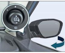
To fold / unfold the ORVMs, keep the Selector switch in center position (i.e. neither 'L' nor 'R, position) and then toggle down. This will operate when the ignition switch is in the "ACC" or "ON" position.
