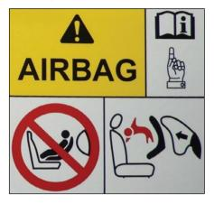
The Airbag Warning Symbol on sun visor reminds of the extreme hazards associated with the use of a rearward-facing child restraint on front passenger seat during airbag deployment. It does not mean that a child cannot occupy front passenger seat and use seat belt. Please refer CRS section for recommended seating positions for children.
