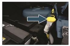
Examine if there is washer fluid in the tank. Fill it if necessary. Use a good quality fluid, diluted with water as necessary.
