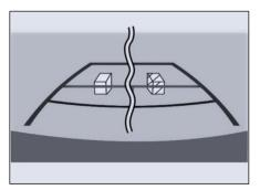
The distance guidelines will appear to be closer to the vehicle than the actual distance.
