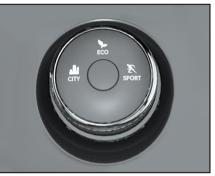
Drive mode selection switch 'ECO ', 'CITY' and 'SPORT' drive modes are provided. These modes can be used to adjust motor torque characteristics and vehicle performance in line with desired requirement.
