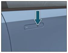
Press the door handle switch (DHS) provided on the driver door to lock/unlock all the four doors except Tail gate.
