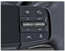
The steering wheel switches are used for ACC operations.
