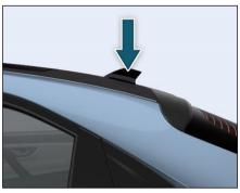
Shark FIN antenna is provided on the roof at rear end.
