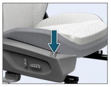
It has 3 ventilation adjustment in decreasing order and LED glows for each press. To stop the ventilation long press the button for few seconds.
