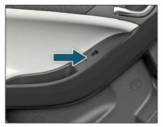
To close the glass pull the switch in upward direction.
