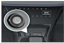
The power socket will work when the ignition switch is in the "ACC" or "ON" position. This socket can be used to provide 12V (10A) power for electrical accessories.
