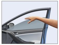
The Anti-pinch function will stop window upward movement if any obstruction or resistance detected.
