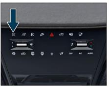
1. Press switch on fascia switch to close charging flap.
