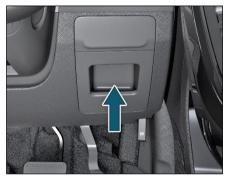
2. To remove the cover, gently pull the cover from upper side that the lugs get disengaged.
