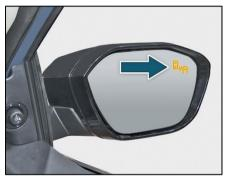
1. When outside rear view mirror warning light is not working properly, the "ORVM indicator failure. Rear ADAS feature Impacted. Please contact service centre" message will appear on the cluster for several seconds
