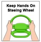
Second instant warning - After taking hands off steering wheel – amber coloured graphic prompting the driver to hold the steering wheel, accompanied by a continuous audio alert.
