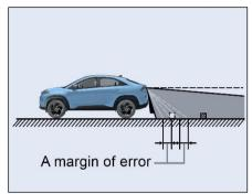
When any part of the vehicle sags due to the number of passengers or the distribution of the load, there is a margin of error between the fixed guide lines on the screen and the actual distance/course on the road.
