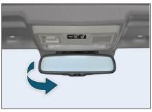
To adjust the mirror move the mirror up, down or sideways manually to obtain the best rear view.
