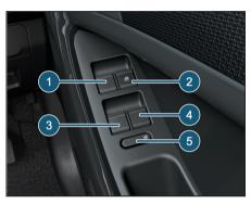
Window glasses 1-2-3-4 on all four doors can be operated by switches provided on the main control panel located on the driver's arm rest. They work only when the key is in the 'IGN ON' position.
