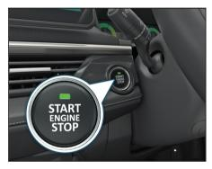
Single press start/stop switch will bring the vehicle to the ACC ON condition (Amber colour)
