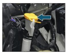
Examine if there is washer fluid in the tank. Fill it if necessary. Use a good quality fluid, diluted with water as necessary.
