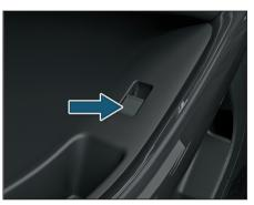
To close the glass pull the switch in upward direction.
