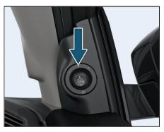
The switch to adjust the motorized mirrors is located on the driver's door. You can adjust the mirrors when the ignition switch is in the "ACC" or "ON" position. To adjust the Mirror
