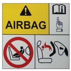
The Airbag Warning Symbol on sun visor reminds of the extreme hazards associated with the use of a rearward-facing child restraint on front passenger seat during airbag deployment. It does not mean that a child cannot occupy front passenger seat and use seat belt. Please refer CRS section for recommended seating position for children.
