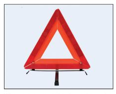
When you press the hazard warning switch, all turn signal lamps will start to blink. Keep the warning triangle at an approximate distance of 50-150 m behind your vehicle in the same lane of traffic. The reflecting side of the triangle should face the oncoming traffic and it should be free
