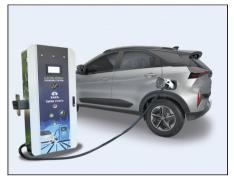
12. Normally the car starts automatically charging. If not, please refer Charging Gun's Fault Indication & Indication Priority Table on the charging station.
