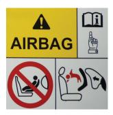
The Airbag Warning Symbol on sun visor reminds extreme hazards associated with the use of rearward-facing child restraint on front passenger seat during airbag deployment.
