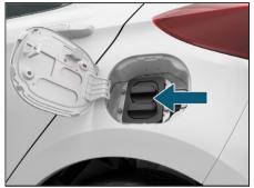
Before connecting the charging gun to vehicle charging socket, make sure the gun lock is released.
