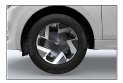
Put a piece of cloth between the spokes of the wheel cover and pull it outwards. Take out detached wheel cover from the wheel rim
