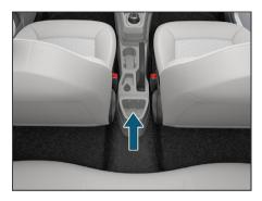
Stowage for the rear passenger is available on rear side of floor console between the front passenger seats. It can be used to keep phone and small items.
