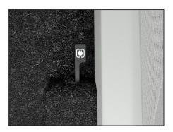
To release the Charging port flap, pull the lever located at the right hand side below the driver seat.
