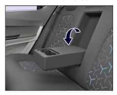
A foldable arm rest has been provided in the rear seat. It also has two cup holders, which can be accessed by opening the cover. When not required, fold the armrest back into the seat.
