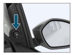
To fold / unfold the ORVMs, keep the Selector switch in center position (i.e. neither 'L' nor 'R, position) and then toggle down. This will operate when the ignition switch is in the "ACC" or "ON" position.
