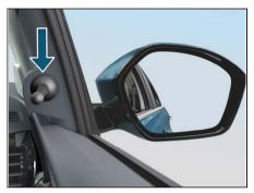
You can adjust the outer rear view mirror manually by joy stick knob located in the driver's and front passenger's door panel.
