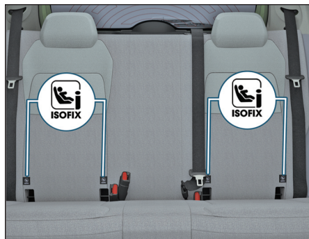
ISOFIX with mounting eyelets
