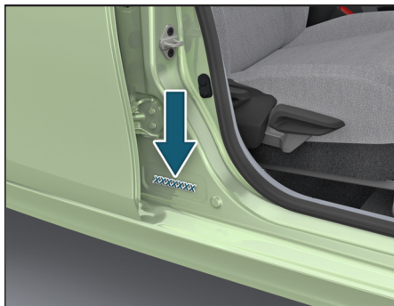
Chassis No. punching near driver seat
